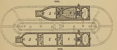
tion of the fuel into the fireplaces  $b^1$ ,  $b^{11}$ , which heat the compartments 2 and 3. The front compartment is heated by the furnace b, which is supplied with fuel through the door f. The several furnaces or fire-places may be provided or not with gratebars as required. g is an airflue extending beneath the floors of all the compartments excepting the last of
